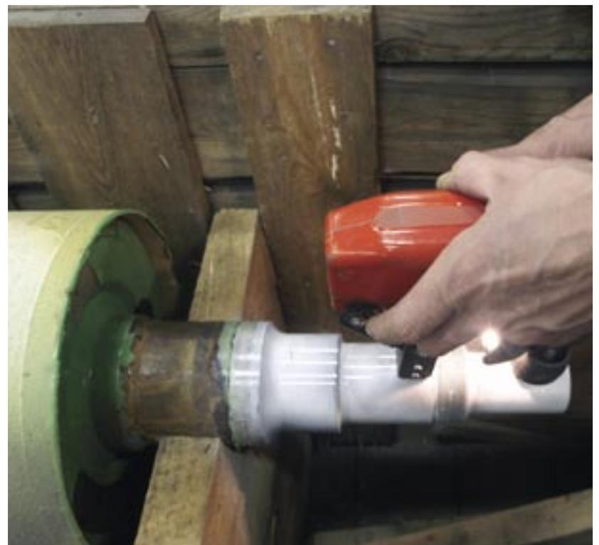
None destructive testing – crack indication.
