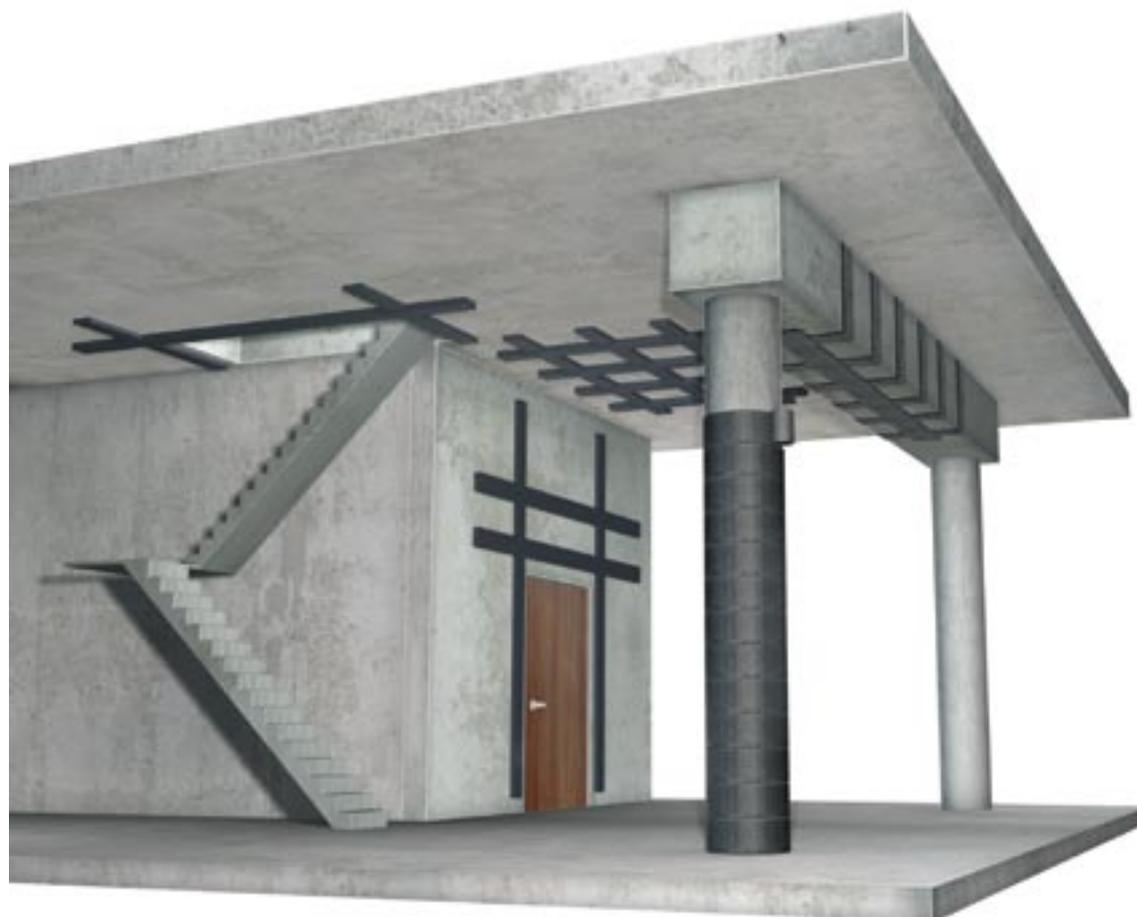
*The illustration shows where carbon fibre composites can be used to strenghtening concrete constructions.*
