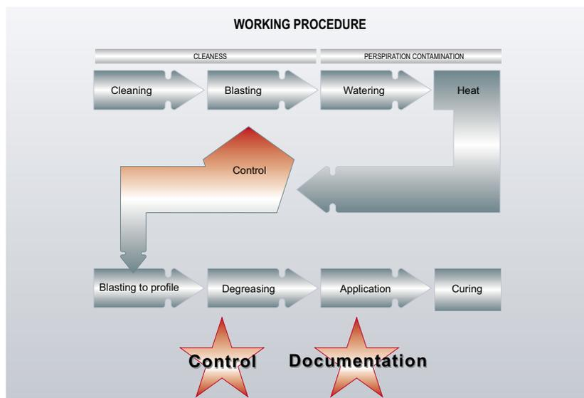
To attain the best possible repair and upgrade of the equipment, the preparatory application and hardening MUST be carried out correctly. To ensure that the work is done properly the whole process is documented.
